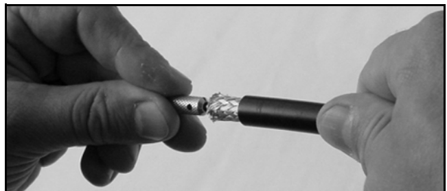
Figure 86: Deburring the Center Conductor
