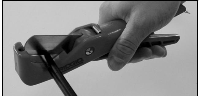
Figure 79: Cutting the Cable
