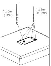
Take the mounting card from the packaging and fold to create installation jig.
