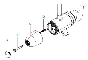
5 Check the O-rings on the nose cone bolt, Active Imaging™ 3-in-1 nose cone and trolling motor lower unit to make sure they are in usable condition and properly installed. If they show damage (cracks, rough edges, voids or discoloration), discard and replace with the supplied O-rings.
