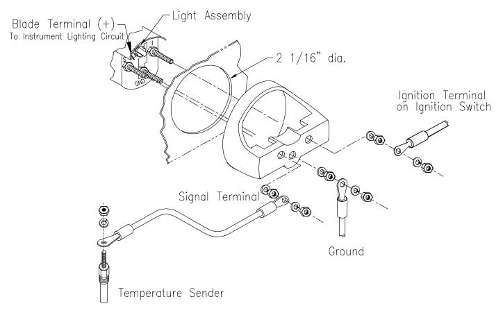
**CAUTION:** Disconnect the battery during installation. Tighten nuts on the backclamp only slightly more than you can tighten with your fingers. Six inch-pounds of torque is sufficient. Overtightening could result in damage to the instrument and may void your warranty.
