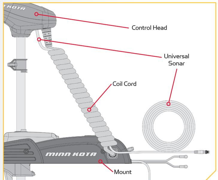
**NOTE:** After the Universal Sonar Cable exits the Coil Cord, it should be routed through an established routing system on the boat, in an area with minimal interference. Inspect the selected route carefully to ensure that there are no sharp edges, obstacles, or obstructions that may damage the cables.
