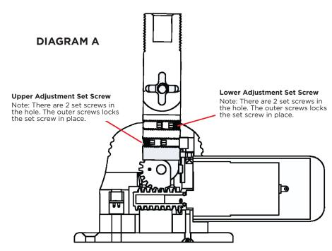
Adjustments to the arm position need to be done slowly 1/4 turn at a time. It is best practice to use an amp meter to determine when the sensor switch disables motor power. Failure to do this could result in motor failure.
