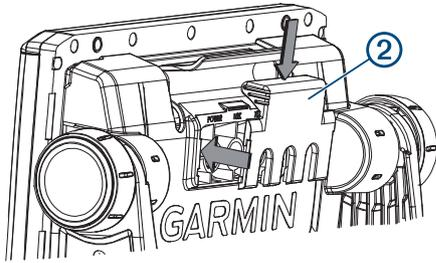
There is an audible click when the locking bracket is installed correctly.
