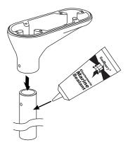
Apply marine adhesive sealant to the mounting holes. Then insert the two plastic rivets into holes as shown.
