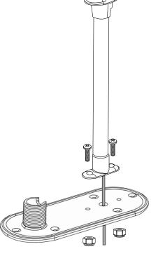
Apply marine adhesive sealant into the groove as shown.
