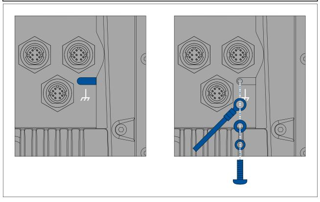
Use a small flat blade screw driver to remove the cover over the grounding screw hole.
