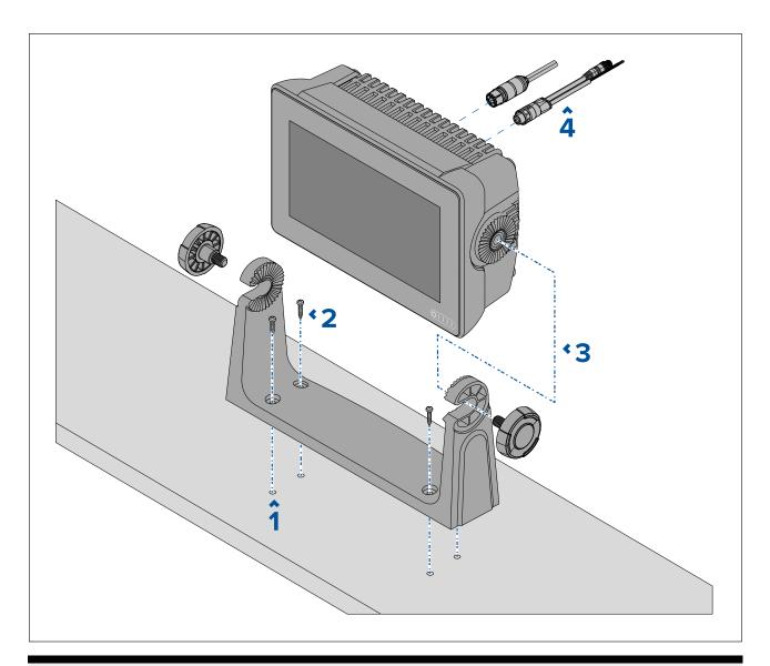
**Note:** The illustration depicts an Axiom<sup>™</sup> 7 being mounted on a plastic trunnion bracket. The trunnion bracket supplied with the Axiom<sup>™</sup> 9 and Axiom<sup>™</sup> 12 are made from metal and so look different than the trunnion shown. A metal trunnion bracket is also available for the Axiom<sup>™</sup> 7 as an accessory; Part number: R70524.
