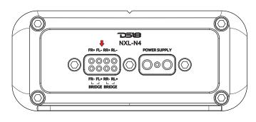
and insert them into the block terminal while being careful that there is no loose or frayed strands of wire and tighten the Allen head screw down on the terminal till the wire is tightly secured in place. If the wires ever come in contact with each other the amplifier will go into protection.
