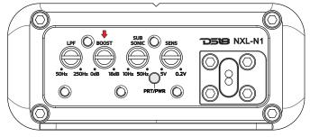
Use Bass Boost carefully. The demands on power output are tremendous. Try to minimize the use by changing woofer position or the enclosure size.
