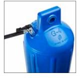
STEP 3 - Fill the Polyform fender or buoy until the walls are fully expanded. The best way to check that is to measure the circumference of the particular product and match the chart measurement. You should also be able to easily push with your thumb and depress the wall 1/4 inch.
