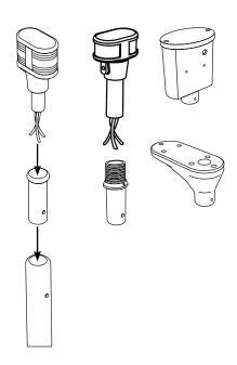
Insert the four nuts into the adapter plate. This has most likely been done for you.
