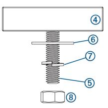
**10** Using a torque wrench, tighten the nuts to 13.7 to 18.6 N-m (10 to 14 lbf-ft.).
