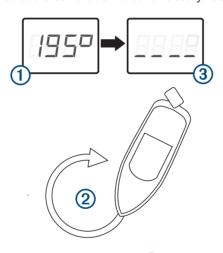
6 Within three minutes, complete two full, slow, tight circles 2, taking care to keep the boat as steady and level as possible.
