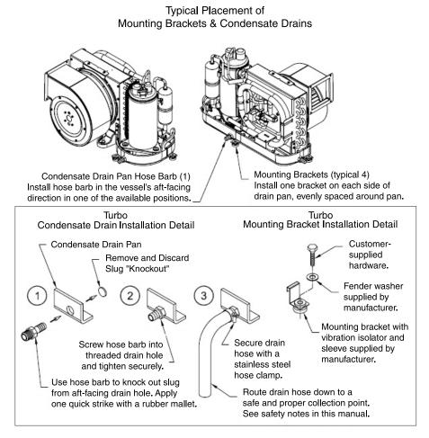
Figure 5: Mounting Brackets and Condensate Drains on Other Self-Contained Systems
