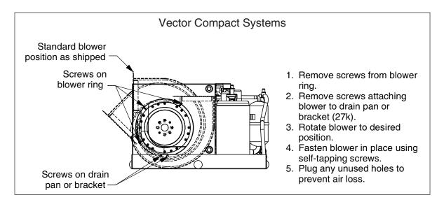
Figure 3: Placement Relating to Airflow
