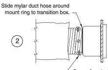
Screw 3 or 4 stainless steel screws through mylar duct hose into mount ring, capturing 2 or 3 wires with screw heads.
