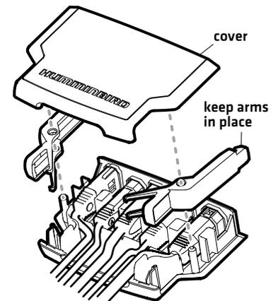
**Connecting the Cable Tray to the Control Head**
