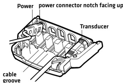
**CAUTION!** It is important to place the connectors into the correct slots and right side up. See the illustration *Locating the Cable Tray Slots* for details.
