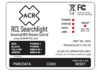
The Wi-Fi Module has an NMEA0183 input that allows an external GPS to provide position information for display in the ACR Searchlight App. This is particularly useful if the mobile device does not have an internal GPS, such as a Wi-Fi only iPad.
