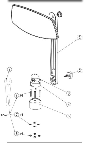
TIP: After tightening the knob in step 10, you can rotate the mirror arm clockwise even further (in the same direction as the knob) to ensure a more secure fit.
