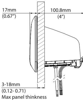
2 Cut the mounting hole and drill pilot holes using the paper template.
