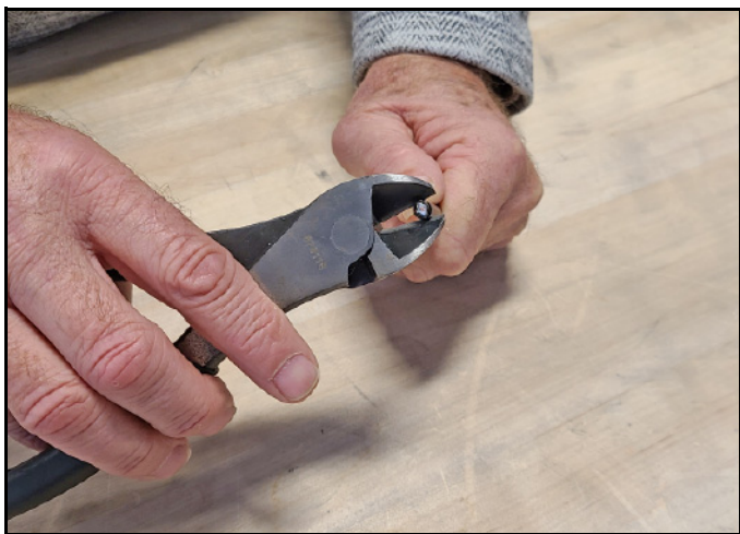
Figure 60: Reshaping the Cable
