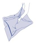
**4** Tension the batten and force the tip in the corner pocket.
