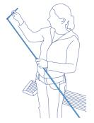
3 Guide the battens through loops and seat in each corner. Make sure the battens are crossed.
