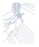
**3** Screw the small white and Blue Performance hooks in place, using the countersunk screws provided.
