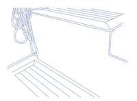
**2** Using the drill pattern supplied drill four 3mm holes in the boat for each corner position.
