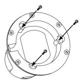
Place the FLIR camera on top of the ADA-F3 top plate. Make sure that the six holes on the adapter line up with the six holes on the top plate.
