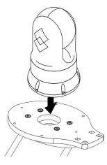
Secure the adapter to the ADA-F3 top plate using the provided two #12 x 1" screws with a philips head screwdriver (one forward and one aft). For the remaining adapter holes you will thru-bolt using four of the M6 x 45mm screws, washers and nuts. Two of each used on each side.
