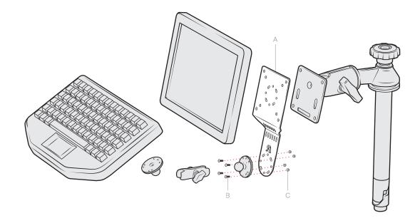
The RAM® Accessory/Display Bracket supports mounting third party keyboards below the monitor, as well as mounting a phone dock or other peripherals beside the monitor. To accommodate multiple peripherals, more than one display bracket may be used.
