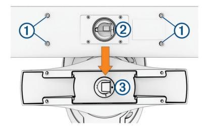
3 Align the waveguide ② on the pedestal with the socket on the bottom of the antenna ③, and slide the antenna onto the pedestal.
