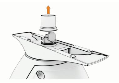
2 Remove the mounting hardware from the bottom of the antenna ①.
