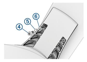
5 Using a torque wrench, tighten the hex screws to 0.81 kgf-m (70 lfb-in. [6 lbf-ft.]) to fasten the antenna to the pedestal without damaging the antenna or the mounting hardware.
