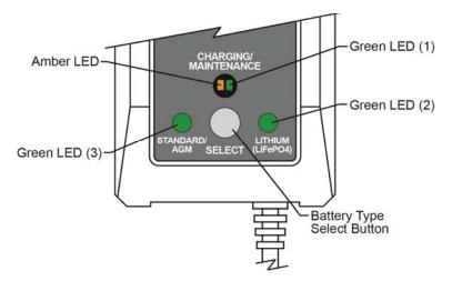
When AC power is first applied to the charger all of the LED's will illuminate for two to three seconds before starting the charge sequence listed below.
