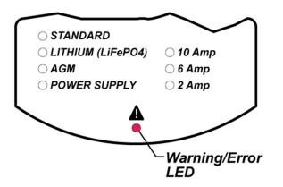
9) NO BATTERY CONNECTION: If there is either no connection or a bad connection between the alligator clips and the Battery, one of the Battery Chemistry LED's will flash and one of the Charge Rate LEDs will be solid and the Battery Level LED's across the top of the charger will also flash.
