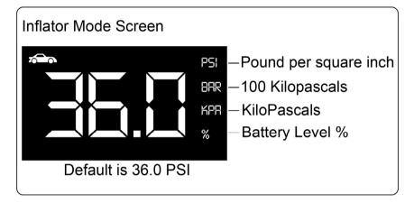
5) The default setting is 36.0 PSI. To change from PSI/BAR/KPA simply press the "Inflator mode" button with a single press.
