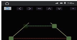
Touch and drag a square icon to reposition the related guide line. Repeatedly touch an arrow icon to fine tune positioning of the related guide line. Touch the OK icon to confirm the adjustment. To reset to the default positioning of the guide lines, touch the Reset icon.
