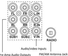
Pre-Amp Audio Outputs FM/AM Antenna (Front/rear speaker outputs and two subwoofer outputs)
