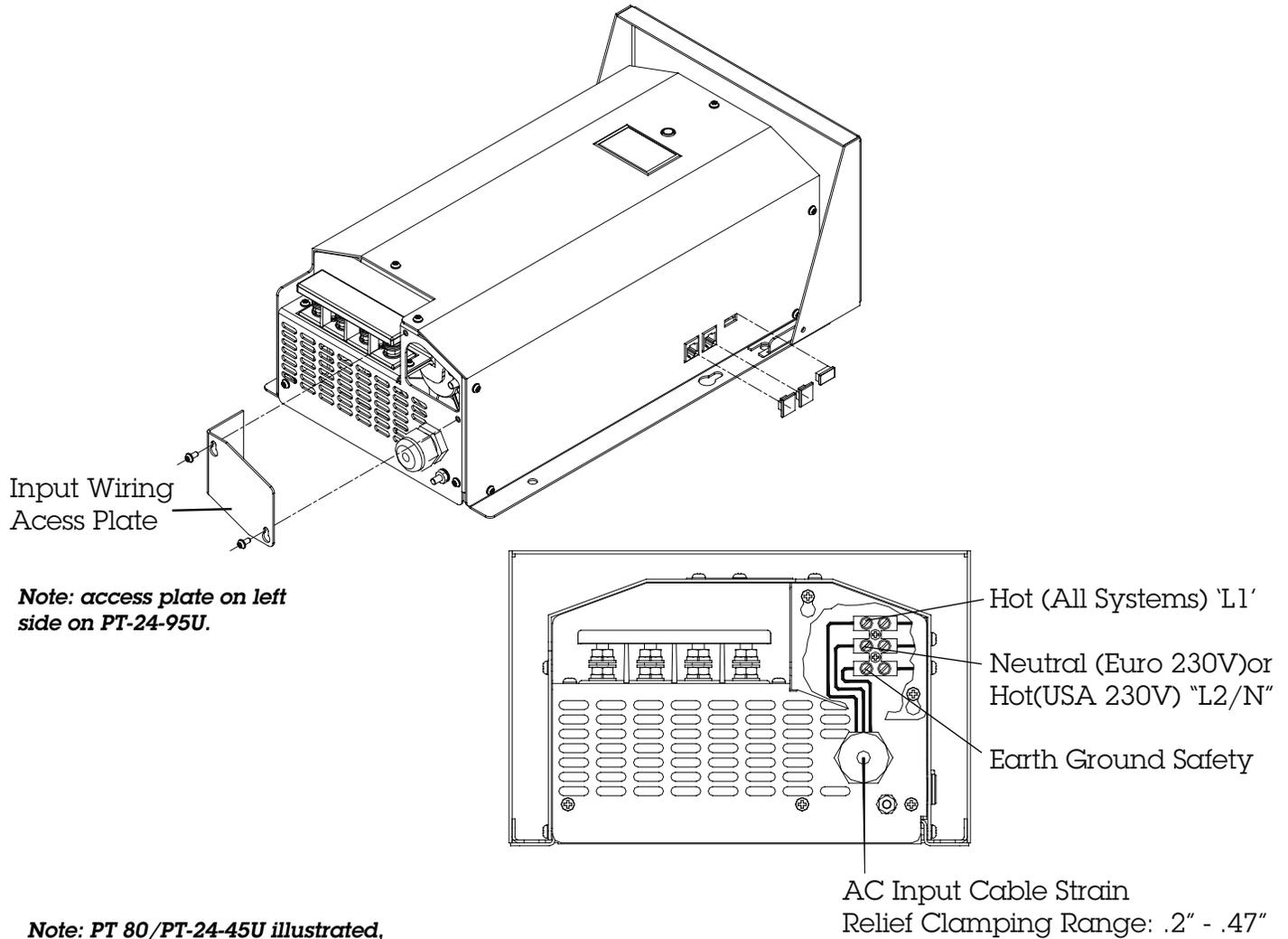
**Note: PT 80/PT-24-45U illustrated, same wiring configuration applies to PT-24-95U, but access plate is on left side.**
