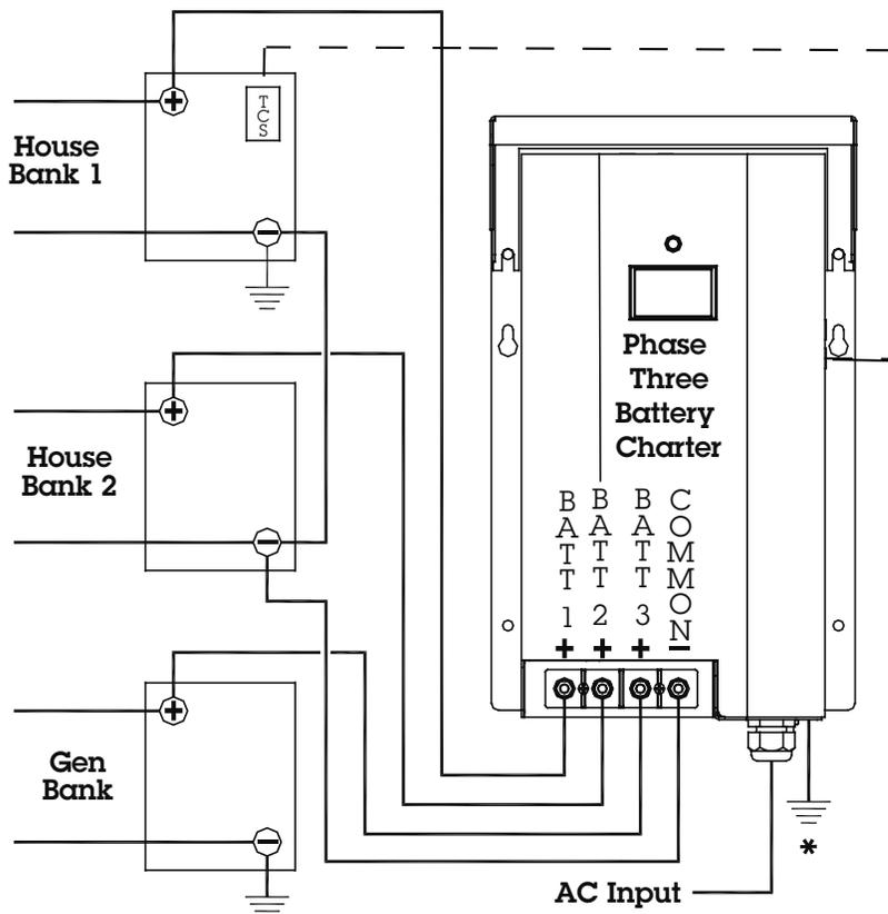
**Optional Temperature Compensation Sensor** See page 9 for installation information. Use provided cable clamps to secure probe cable
