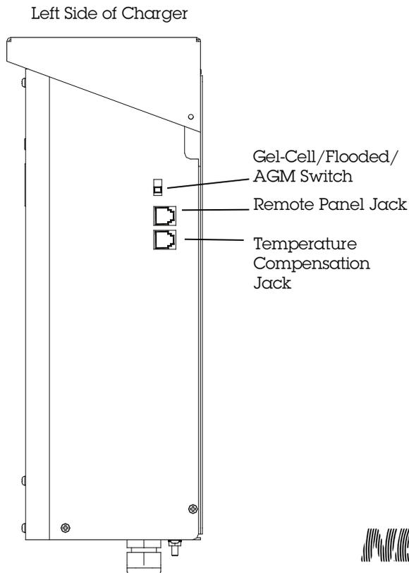
**section III-E) and using the temperature compensation option, you must use a separate sensor for each charger, and the sensors must be mounted close together in the same battery box or on the same battery for proper operation.**
