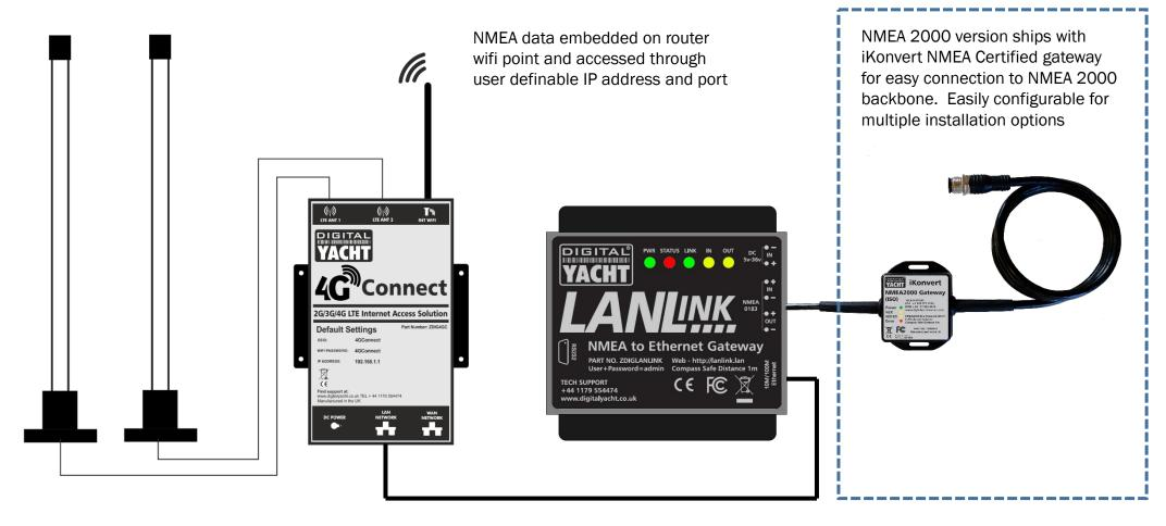
Simple ethernet patch cable connection to router
