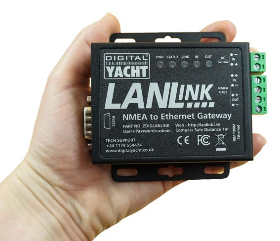
LANLink is available in two versions suitable for NMEA 0183 and NMEA 2000 respectively. It features an easy to use web interface allowing any device with a browser to configure NMEA baud rates and IP/Port information.
