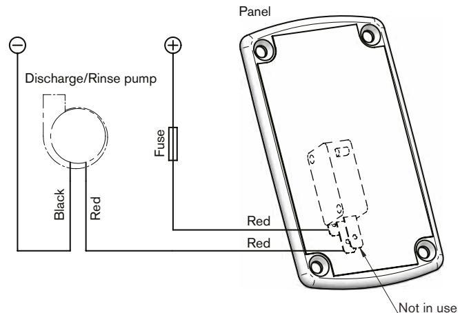
Panel Red (upper wire on switch) to positive (+) battery via one fuse
