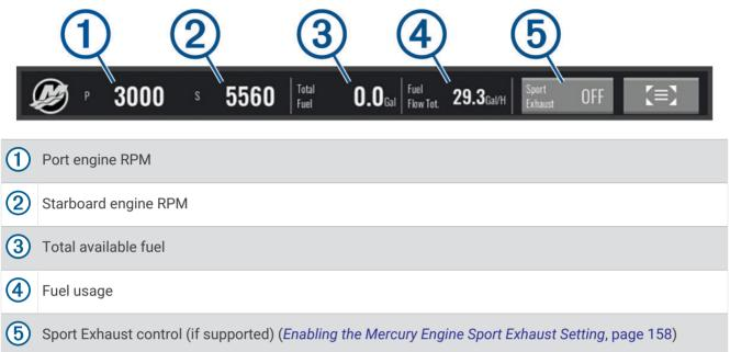
**TIP:** You can also view an overview of engine details on the Mercury gauges page (*Mercury*<sup>®</sup> *Engine Gauges*, page 143).
