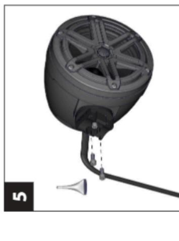
Apply Loctite® red thread-locking compound to two M6 x 16 mm Machine Screws, slide them through the slots in the clamp receiver, into the appropriate holes in the fixture base, and fully tighten.
