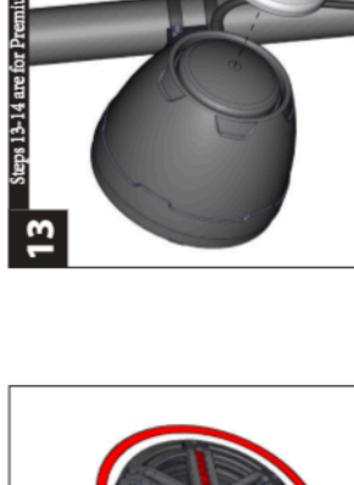
Clean the inside of the aluminum cap with acetone (not included) prior to attaching it to the enclosure. Apply a circular head of silicone adhesive to the inside of the aluminum logo cap. 1/2-inch (13 mm) from the outer edge.
