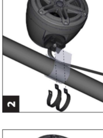
Place the supplied plastic strip around the pipe to prevent scratching. Push the clamps over the pipe (remove the plastic strip). Align the clamps with the clamp receiver on the enclosure.
