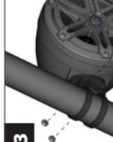
Secure the clamps to the clamp receiver using a pair of M6 x 16 mm Machine Screws, M6 Flat Washers, and M6 Locknuts as illustrated. The locknut should be installed into the hex shaped recess on one end of each clamp. Hand-tighten, allowing just enough freedom to rotate the enclosure around the pipe.
