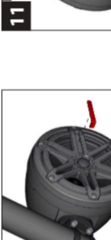
Remove the backing from the rear logo applique. With the logo positioned at the desired angle, attach the applique to the back of the enclosure.
