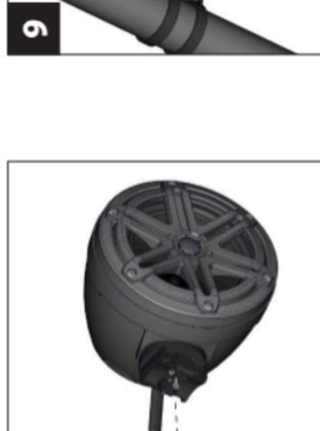
If you wish to rotate the speaker's grille/logo badge alignment, remove the six #8 x 1-1/4" speaker mounting screws and #8 Flat Washers.
