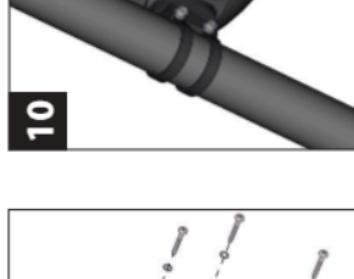
Rotate the speaker to the desired angle. Reinstall the speaker and speaker mounting screws and washers. Hand-tighten in a criss-cross pattern.
