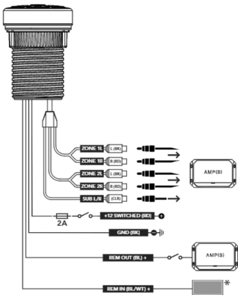
\* Optional connection to a source unit's remote turn-on output (+12V). If used, the MBT-CRXv3 power button will no longer operate.
