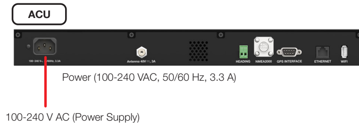
Figure 24: Connecting Power to ACU
