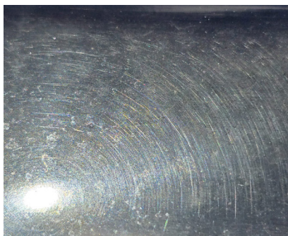
Image 2.1: Surface with scratches/swirl marks.
