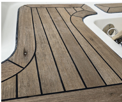
Image 4.3: Dirty teak in heavy traffic area. Needs heavy cleaning.
