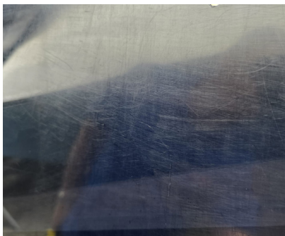
Image 6.5: Heavily scratched glass.
