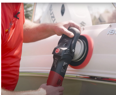
Image 2.2: Paint correction using compounds and a dual-action polisher.
