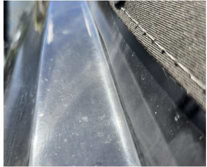
Image 2.3: Swirled and sun faded paint.
