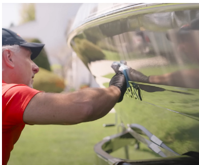
Image 3.4: Due to quick flash times, it is recommended to apply ceramic coatings in small sections.
