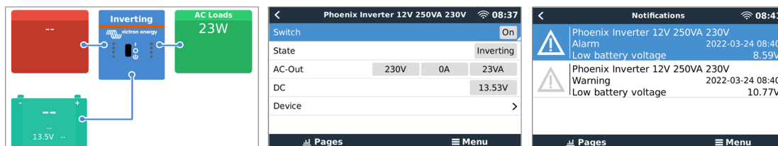
Example of GX screens from left to right: system screen, inverter device screen and an alarm message.
