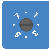
Rotary switch set to position 2
