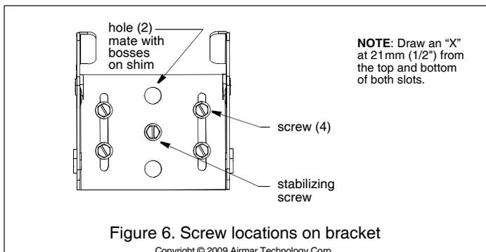
5. Using the vertical adjustment space in the bracket slots, slide the assembly up or down until the bottom inside corner of the transducer projections 0–3mm (0–1/8") below the bottom of the hull (see Figure 1). When you are satisfied with the position of the transducer, tighten the four bracket screws. For clear access to the screws, remove the transducer assembly from the bracket (see Figure 4). *When reattaching, be sure to include the spacer.*
