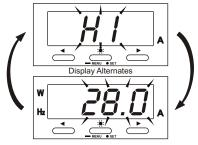
The alarm system is capable of recognizing more than one alarm condition at a time. If more than one alarm is set, the meter will continuously check for each alarm condition. If an alarm condition occurs while in scan mode, or while displaying a different parameter, the display will shift to the alarm value.
