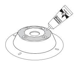
Apply marine adhesive sealant to the inside of the four bolt holes on the top plate.
