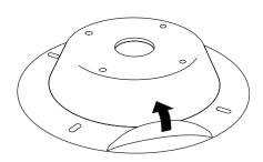
Apply marine adhesive sealant to the base of the mount. Be sure to go around the base holes.
