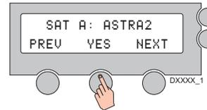
1. Follow steps 1 thru 3 for entering set up mode. Press YES to set satellite pair.
