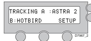
2. Antenna is tracking Satellite A
