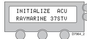
1. Communication is being established between the antenna and the ACU.
