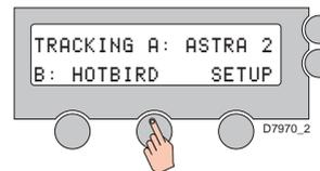
4. Antenna is again tracking satellite A. Press center soft key to display position detail.
