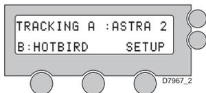
4. The antenna has located the satellite and is now tracking.
