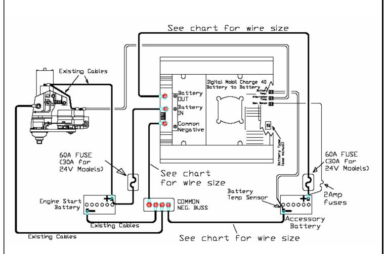
**Wiring:** Connect all wiring with fuses removed from wiring fuse holders to protect against accidental shorting and the units Sleep and an Auto Start feature. If the input voltage (engine start battery) is above 13 volts for 12V models (26V for 24V models), then the unit will auto start. Ensure all wiring is correct before re-inserting wiring fuses.
