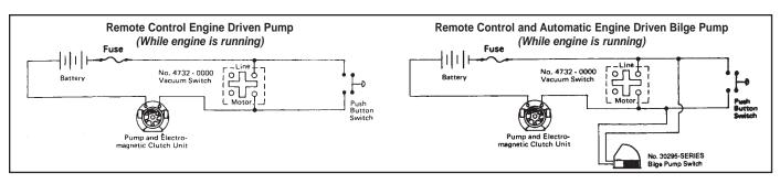
**REMOTE CONTROL:** Install a pushbutton switch at one or more locations (multiple switches should be wired parallel). Depress pushbutton for 2 seconds. If there is water in bilge, pump will operate until dry, at which time vacuum switch will stop pump. If no water is in bilge, pump will stop when pushbutton is released.
