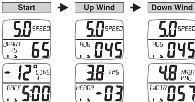
Programming these pages into the Autoleg Page prior to the race would automatically show these pages for the appropriate leg of the course; leaving the tactician free to concentrate on the race, not on configuring his instruments.
