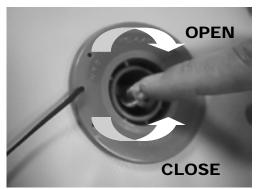
To open valve, depress stem and rotate clockwise. To close valve, depress stem and rotate counter-clockwise.
