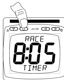
Press to resynchronise to nearest full minute (8:00)
