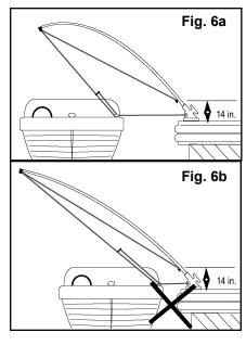
Under no circumstances should any mooring whip installed with an excess of tension as shown in thesediagrams. Doing so will affect the mooring whips ability to protect your water craft and will void the manufacturers warranty.
