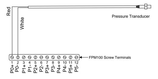
Figure 1 – Pressure Transducer Connection Diagram
